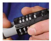
Press snap-in button. Turn the handle and push to required position until the arrow point is visible in the opening. Turn handle back and click into place.
