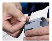
Before inserting the support connector, remove the strap without using a tool.
