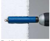
The drilling depth stop ensures that only the amount of insulation material is removed which is necessary to secure the mini equipment carrier.
