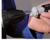
TIP: To cut several openings or work with hard plastic, you can fit the opening cutter on the 1/4" bit of a battery-powered drill.
