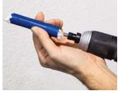
By simply unscrewing the cutter head, the drilled core can be removed quickly using a centering drill.
