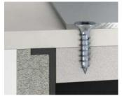
Use only screws that go into but not through the mineral fibreboard when attaching the device! (e.g. SPAX countersunk head screw 3.5 x 15 mm)!
