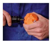
Push the point into the housing and cut out required opening by turning to the right.
