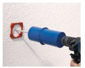
The centering aid Ø 68 mm and depth stop on the cutter ensure a precise opening without damaging the existing cable.
