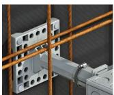
Wall thickness up to 20 cm: Shorten the 8-sided tube at the base plate and the support plate to the appropriate length. Wall thickness 20 to 25 cm: Adjust the telescopic support to the appropriate length.
