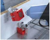
Wall and ceiling transitions for attachment with hot glue.
