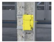
The Flat 45 fixing and support elements for wall thicknesses of 6 to 12 cm press the box front against the working formwork and ensure secure positioning.
