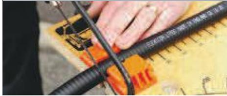
Metallic conduits should be cut with a fine tooth (32 TPI) hacksaw or bandsaw. Ensure you make a straight vertical cut. Our clamping vice, part no. BSB makes the use of a hacksaw much easier.
