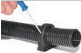
Ensure the hinged lid is open and insert the conduit from above. The clip size is shown on the clip for easy reference. The clip provides a secure fit whether the hinge is open or closed. The FCL clip includes an internal rib to help locate and retain corrugated conduits. The FCL-P clips do not have this rib and can therefore be used with plain or smooth outer conduits.
