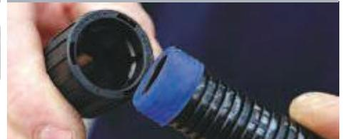
The FPAX fitting features a conduit seal to provide an IP rating up to IP69. This simply fits onto the end of the conduit before the fitting is connected to the conduit. To aid assembly moisten this seal. For a one piece fitting with an IP69 rating use Ultra™ (An FPA fitting cannot be uprated to IP69 with the addition of a seal). Pull back slightly to ensure the locking teeth mechanism has engaged with the corrugations.
