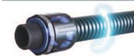
For Ultra™, Flexilok® and FPA fittings simply push the conduit into the end of the fitting with a slight twist until it will go no further. Pull back slightly to ensure the locking teeth mechanism has engaged with the corrugations.
