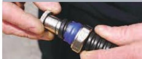
Firstly place the back nut on the conduit followed by the seal (note the orientation). Next, screw the insert into the end of the conduit until this gives a secure fit.
