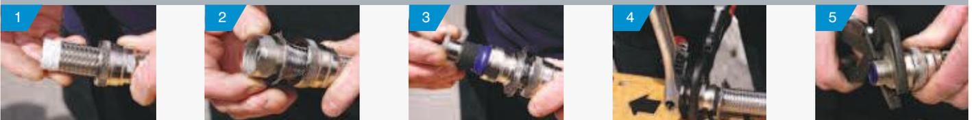
Our type-C braided fittings consist of an outer compression nut, an inner compression nut, an elastomeric seal, an insert and a body. Firstly place the outer compression nut on the conduit as per 1. Remove the tape securing the braid and pull back to allow the inner compression nut to be fitted as per 2. Next, fit the elastomeric seal (note the orientation) and screw the insert into the end of the conduit until this gives a secure fit as per 3.
