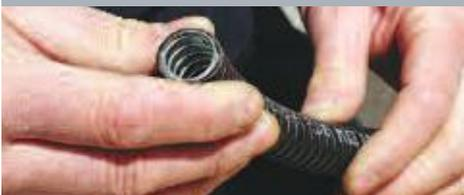
Our fitting's components are supplied part assembled to illustrate how they go together. Our C type fittings consist of a compression nut, an elastomeric seal, an insert and a body.
