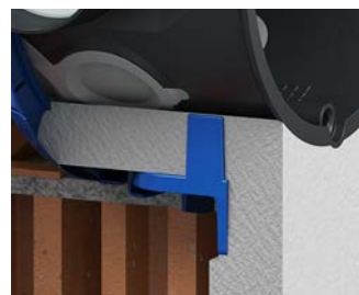
The plaster penetrates up to the lamellar ring and thus ensures that the box is securely and permanently fixed.
