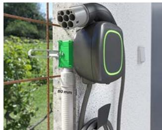
Thanks to the conduit transition coupling  $\varnothing$  32 mm (Art. No. 1263-32), the one-gang junction box Flat 45 can be used as a wallbox junction box in walls from 75-80 mm.
