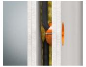
Bending of the conduit up to 90° is easily possible in the case of slim wall constructions or in the installation level.
