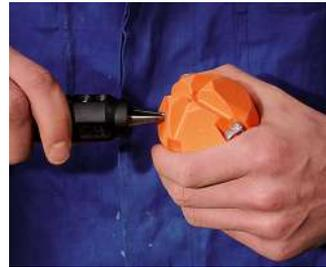
Push the point into the housing and cut out required opening by turning to the right.
