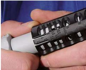
Depending on the use, find the required diameter in the corresponding table and locate on tool.
