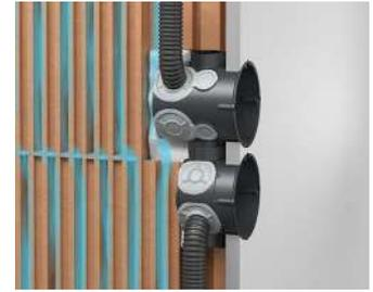
Vertical draughts occur in hollow chamber blocks. The UP boxes with ECON® technology prevent air exchange.
