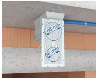
Universal front part for installation diameter of  $\varnothing$  68 mm for knocking in or universal up to  $\varnothing$  86 mm for cutting out (turn by 180°).
