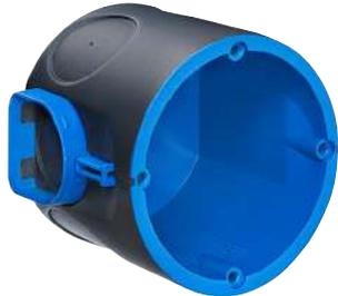
The flush-mounting sound insulation box offers 6 possible entries for conduits up to M25 and cables up to Ø 11.5 mm.
