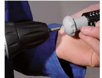
TIP: To cut several openings or work with hard plastic, you can fit the opening cutter on the 1/4" bit of a battery-powered drill.
