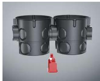
Plug the one-gang junction boxes together and insert the tunnel connector (item no. 1159-36) between the two one-gang junction boxes...
