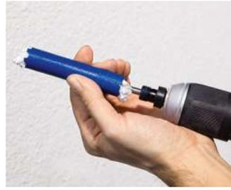
Release the cutter head and remove the drilled core.
