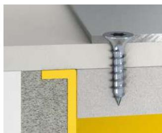
When attaching the device to the installation housing, use only screws that go into but not right through the mineral fibreboard cover (e.g. SPAX countersunk head screw 3.5 x 15 mm)!
