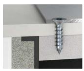
Use only screws that go into but not through the mineral fibreboard when attaching the device! (e.g. SPAX countersunk head screw 3.5 x 15 mm)!
